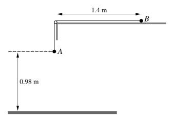
Particles A and B have masses 0.32 kg and 0.48 kg respectively. The particles are attached to the ends of a light inextensible string which passes over a small smooth pulley fixed at the edge of a smooth horizontal table. Particle B is held at rest on the table at a distance of 1.4 m from the pulley. A hangs vertically below the pulley at a height of 0.98 m above the floor (see diagram). A, B, the string and the pulley are all in the same vertical plane. B is released and A moves downwards.
